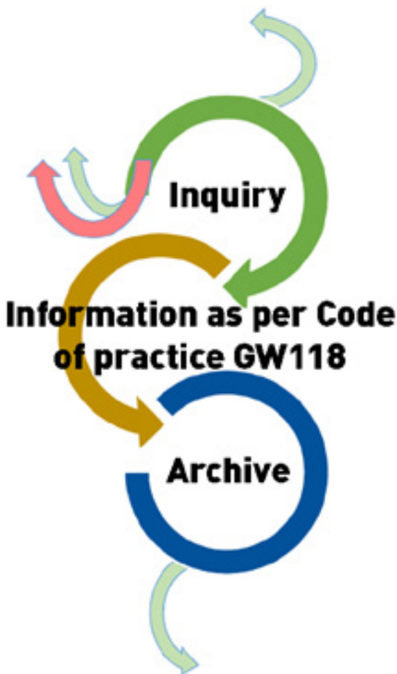
Figure 2: Pipeline/cable inquiry process illustrating the leeway in terms of inquiry and archiving. It can be seen, that only the process to be implemented on the operator side has been standardized by the rules and regulations (code of practice GW118)
