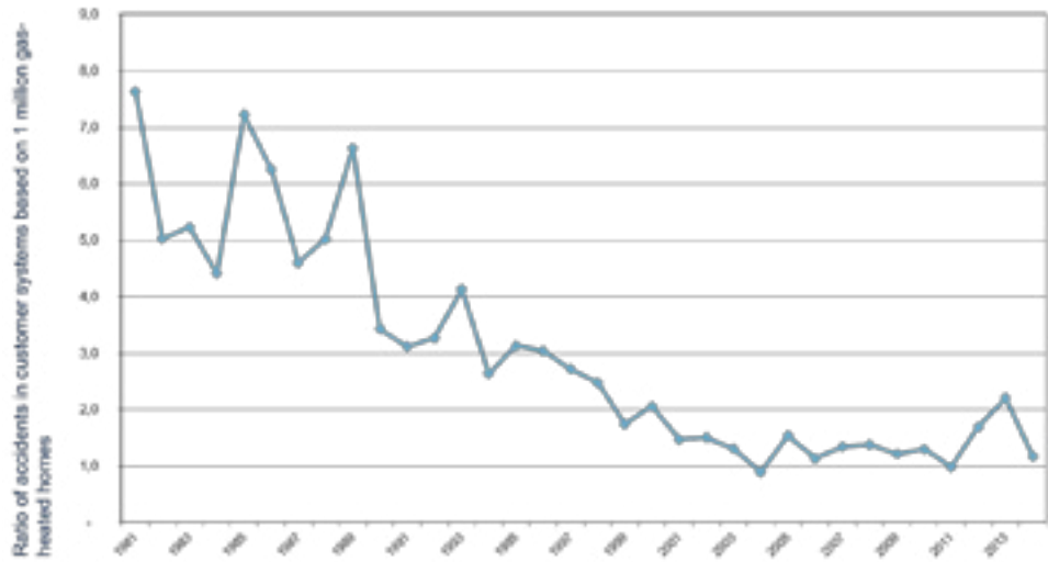
Figure 6: Ratio of accidents in customer systems based on one million gas-heated homes
